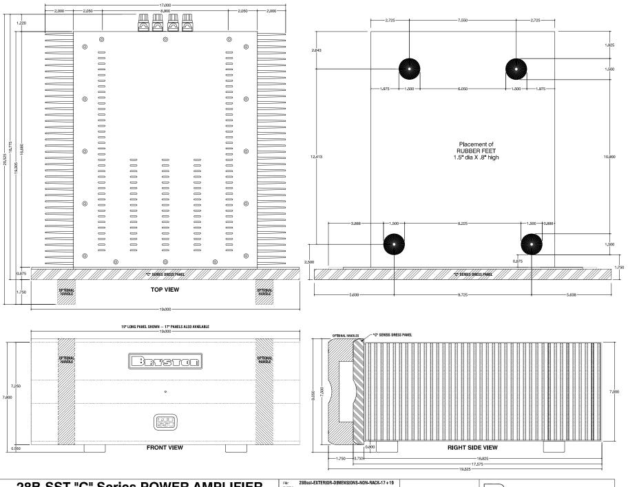
28B-SST "C" Series POWER AMPLIFIER EXTERIOR DIMENSIONS for NON-RACK-MOUNT MODELS
