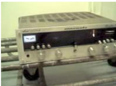
Post relocation to the basement for the final portion of our truncated tank test, Jay Bee plugged the Marantz in and, lo, some of the lights came on. The tuning display remained dark, and as if auguring other malaise within the unit's tuner, it didn't look like it would work; the tuning capacitor's plastic drive assembly was a hopeless piece of junk, its dial cord melted.
