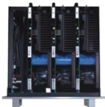
**Modular design with independent power supplies each with its own transformer for precise sound-staging.**
